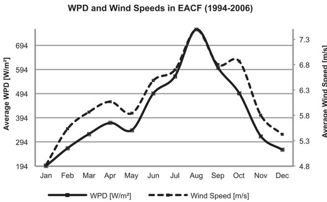
**Fig. 5.** Monthly averages of Wind Power Density (WPD) and wind speeds, 1994–2006. Elaborated based on data collected by CEPTec-INPE [20].
