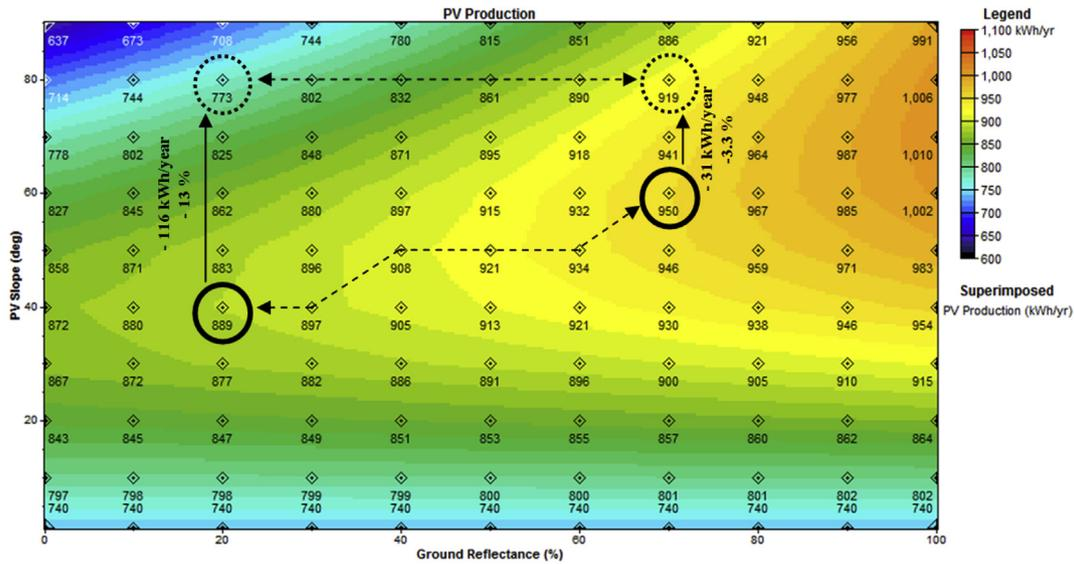
Fig. 3. Influence of ground reflectance in the optimal slope angle of the photovoltaic panel. Simulated for 1 kWp of panels, at 180° of azimuth.
