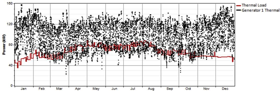
Fig. 11. Production of thermal energy of the power generator, superimposed on the thermal load.
