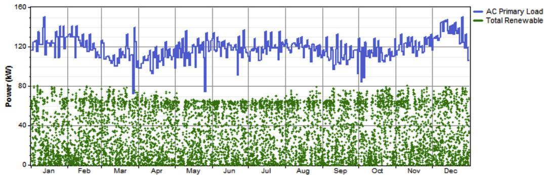
Fig. 9. Hourly AC primary load and renewable generation for the proposed hybrid energy system.
