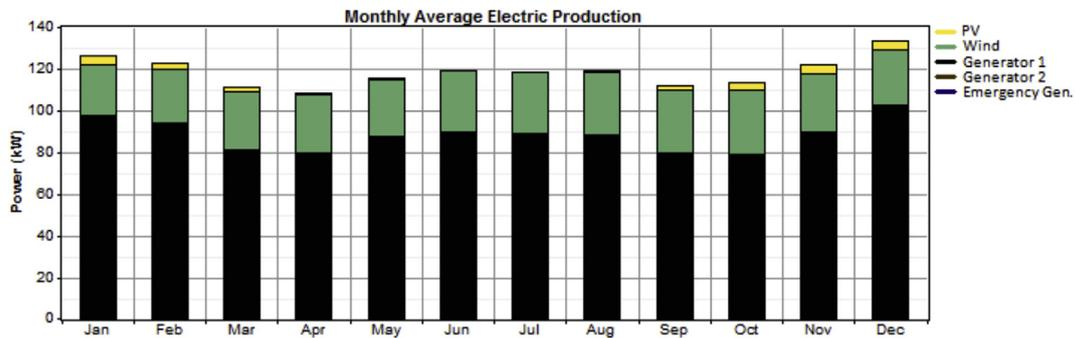
Fig. 8. Monthly average electric production for each technology of generation, for the proposed hybrid energy system.
