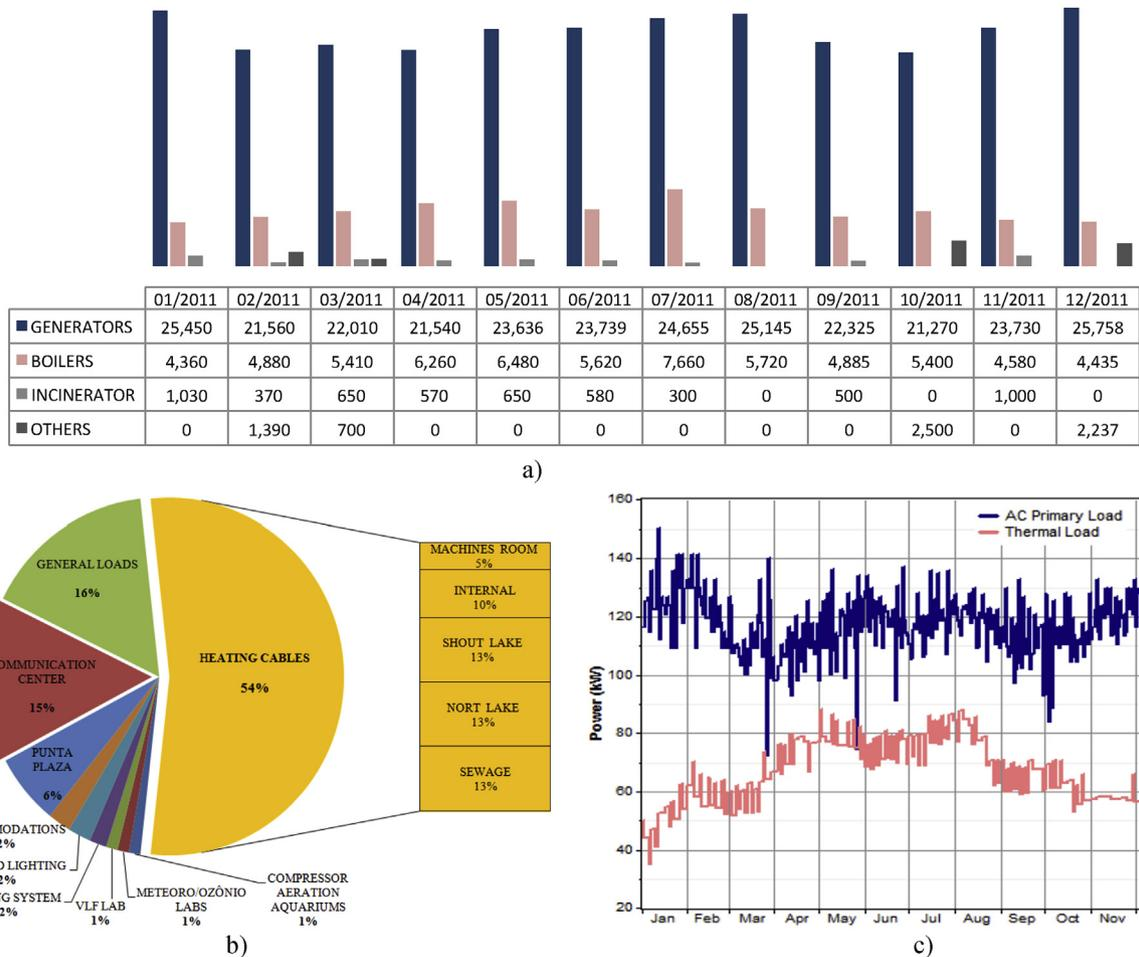
Fig. 1. a) EACF fuels consumption in 2011; b) EACF electric loads profile in 2011; c) EACF average daily demand of electric loads and the heating system demand along 2011.
