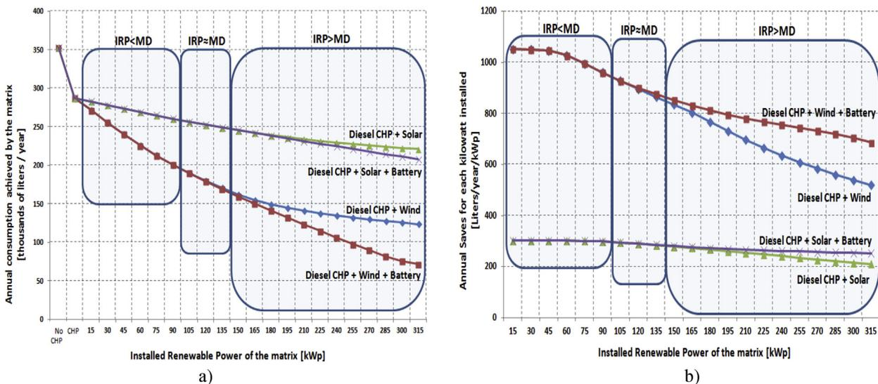
Fig. 7. a) Annual diesel consumption in the Station as a function of the installed renewable power; b) Annual diesel saved per installed kilowatt of renewable, for each matrix configuration.
